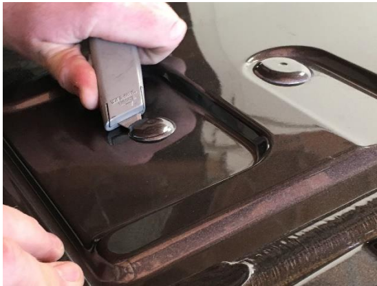
Figure 14: Roof Rack Mounting Point Plug Removal
